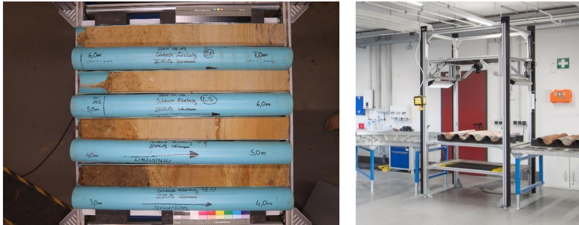
Figure 1. Core sample image obtained from geotechnical site investigation, along with core sample imaging setup housed in a photo box of the BAW soil mechanics laboratory in Hamburg.
